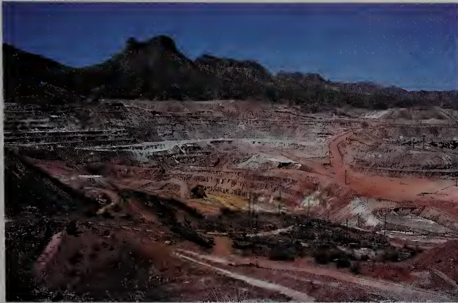
FIGURE 15.39 The Ray Mine, a great open-pit copper mine near Teapot Mountain, Arizona. Because the copper minerals are disseminated through an enormous body of igneous rock, large volumes of rock must be excavated. (Mark A. Melton.)
