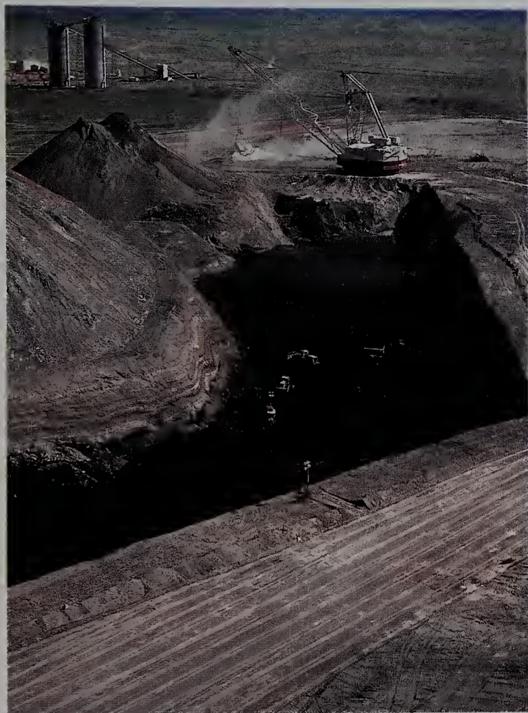
FIGURE 19.17 Strip mining of a great coal seam at the Antelope Mine, Douglas, Wyoming. Overburden is being removed by the huge machine in the distance, while the exposed coal is being removed by machines in the foreground. (Kristin Finnegan/Allstock.)
