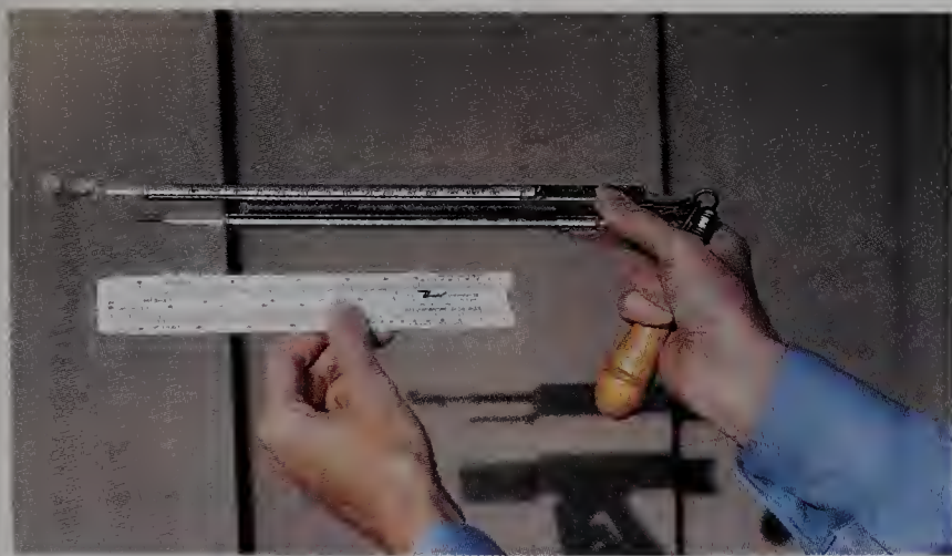
FIGURE 6.5 This standard National Weather Service psychrometer uses paired thermometers. The cloth-covered wet-bulb thermometer projects beyond the dry-bulb thermometer. The handle is used to swing the thermometers in the free air. Below it is a special slide rule that enables rapid calculation of relative humidity from dry bulb and wet bulb readings. (A. N. Strahler.)
