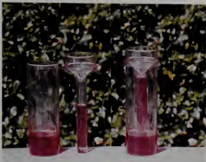
FIGURE 6.15 This 10-cm (4-in.) rain gauge is made of clear plastic, allowing the amount of rain caught in the inner cylinder to be read from the outside. Rain exceeding the capacity of the inner cylinder overflows into the outer cylinder and can be measured after the rain period has ended. (A. N. Strahler.)
