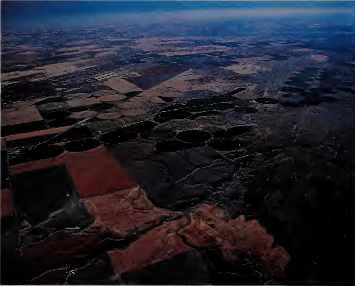
FIGURE 16.27 The perfect circles of green laid out in orderly patterns are thriving plots of food and forage crops—corn, wheat, beans, alfalfa, or grass—irrigated by walking sprinkler systems. Called centerpivot irrigation, the system consists of a long pipe mounted on wheeled supports. The pipe is held fast to a center point where the water is injected and creeps slowly round and round in a huge circle emitting water from sprinkler heads along the pipe. Water is supplied from deep wells close by. (Courtesy of Valmont Industries, Incorporated, Valley, Nebraska.)
