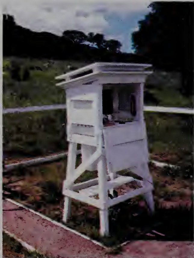
FIGURE 4.1 This instrument shelter houses thermometers and an instrument for measuring relative humidity. (Arthur N. Strahler.)
